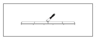
Once the tiles have been glued in place, grout the tile joins and allow to cure.
