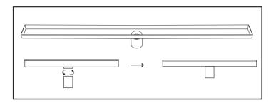
3 Attach a stainless steel spigot to the channel and lock in position.
