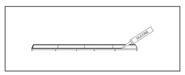
3 Seal around the perimeter of the tile insert (where the tile insert and tiles meet) with silicone sealant and allow to cure.
