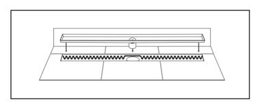
**5** Lower the channel insert into the channel cut-out and allow to cure.
