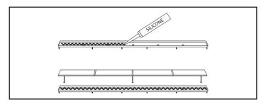
• Glue tiles into the tile insert using silicone and allow to cure.
