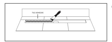
Apply an appropriate amount of tile adhesive or silicon to the channel cut-out.
